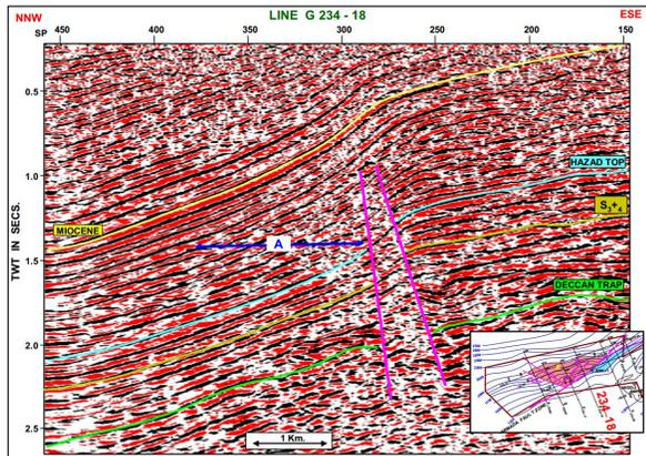
Figure 2: Seismic section displaying the potential zone for CO<sub>2</sub> injection, S<sub>3+4</sub>, from the study area (ONGC India Pvt. Ltd, personal communication).
